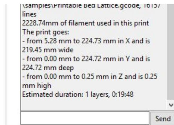
**Console:** Displays feedback from the printer in text Form. Also allow the user to input some G-Code commands manually.
